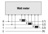
Note that direction of current flow in the current loop must be as shown. Interchange connections to input terminals to simulate flow of **reverse power**.
