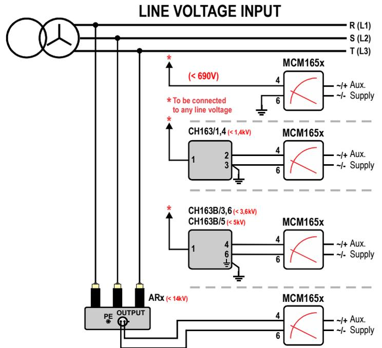
The instrument will detect earth fault on all phases independent of which phase is connected to terminal 4.
