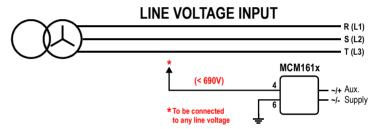
The instrument will detect earth fault on all phases independent of which phase is connected to terminal 4.
