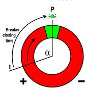
The breaker closure is initiated at "T" when the breaker coil is energised and finalises at "P", assuring a precise "12 o'clock" synchronisation. Allowed frequency difference is adjustable between 0.1Hz to 2Hz. The angle "a" varies according to the frequency difference between the two systems.
