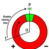
The breaker closure is initiated at "T" when the breaker coil is energised and finalises at "P", assuring a precise "12 o'clock" synchronisation. Allowed frequency difference is adjustable between 0.1Hz to 2Hz. The angle " $\alpha$ " varies according to the frequency difference between the two systems.
