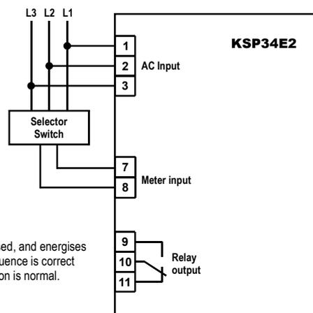
Relay shown de-energised, and energises only when phase sequence is correct and supply condition is normal.
