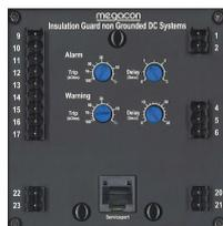
Without any movement of potmeters, the meter will revert to normal Insulation Monitoring Mode after approximately 10 seconds.
