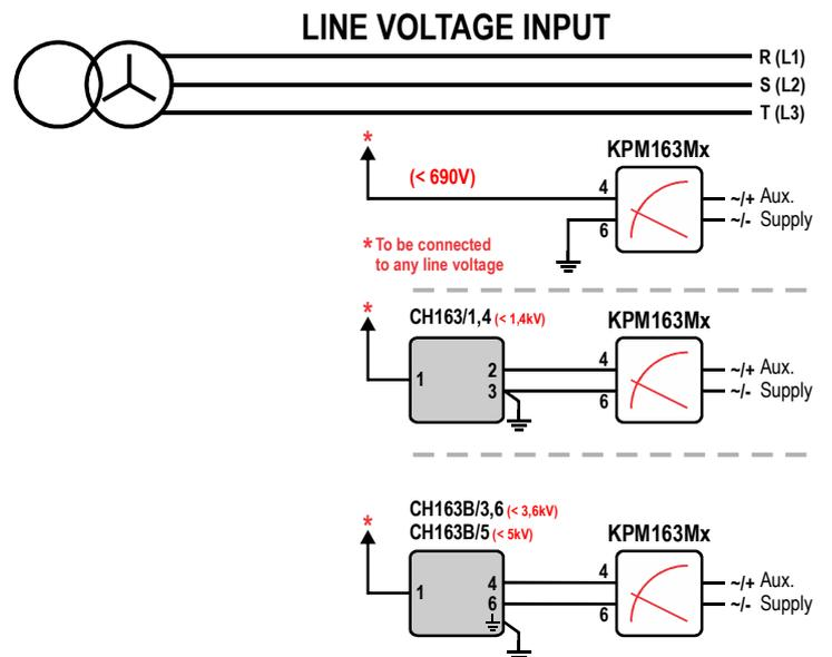
**!** The instrument will detect earth fault on all phases independent of which phase is connected to terminal 4.
