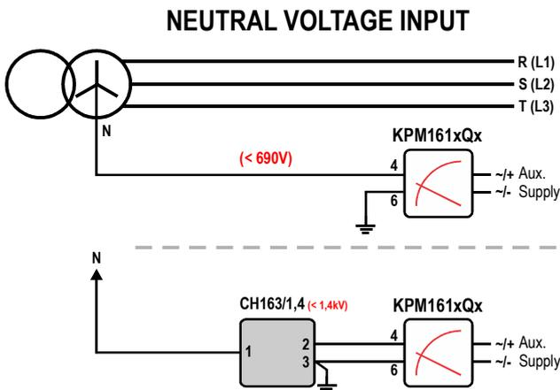
**!** The instrument will detect earth fault on all phases independent of which phase is connected to terminal 4.
