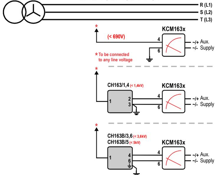
**!** The instrument will detect earth fault on all phases independent of which phase is connected to terminal 4.
