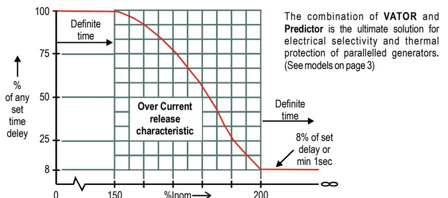
Release characteristic combining definite time and dynamic response to maintain thermal capability protection and selective protection between paralleled generators.
