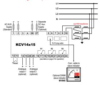
\*Reset: Any latched relay is reset by linking terminals 12 and 13 or by interrupting the auxiliary voltage supply.
