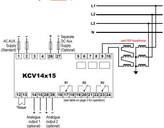
Connection Diagram with optional slave instrument
