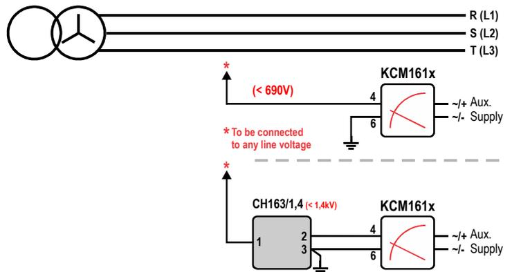
**!** The instrument will detect earth fault on all phases independent of which phase is connected to terminal 4.
