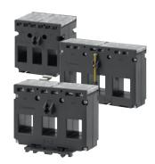
A range of 3-in-1 current transformers combine three traditional current transformers in one moulded case. 3-in-1 current transformers can be directly installed next to a three-phase moulded case circuit breaker, thus saving installation time where fitting three standard individual current transformers would be required. The M3N1 range of current transformers offers primary currents between 60-630A with 5A secondaries with up to Class 0.5 accuracy performance.
